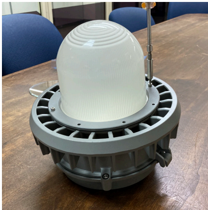
Step 7. If also using the dome guard, replace 4 pcs M4*16 screws, leaving one hole empty between each one. Tighten to 1.47 ft lb. If not using the dome guard, replace all 8 pcs M4*16 screws. Tighten to 1.47 ft lb.
