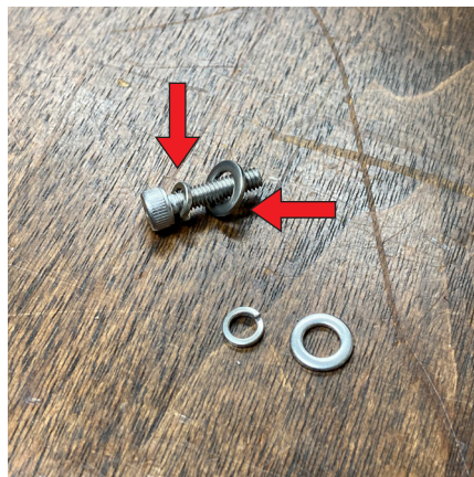
Step 9. Using the remaining 4 pcs M4*16 screws, 4 pcs small locking washers and 4 pcs larger washers (as shown), secure dome guard by tightening screws into 4 remaining holes. Tighten to 1.47 ft lb.
