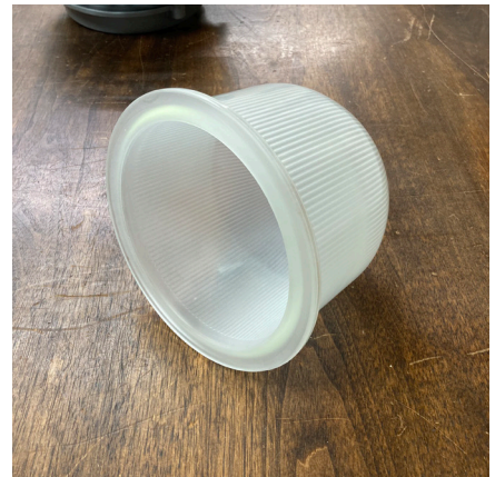
Step 4. Clean dome lens with alcohol wipe.
