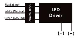
THROUGH-WIRING (NICOR has provided quick-connect wire connectors internal to the luminaire for through-wiring applications.)
