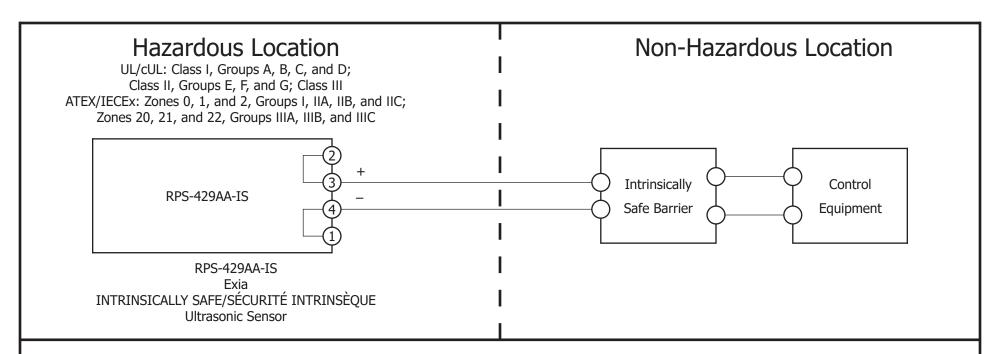
RPS-429AA-IS (4-20mA Analog Current Version) Exia INTRINSICALLY SAFE/SÉCURITÉ INTRINSÈQUE Apparatus Entity Parameters
