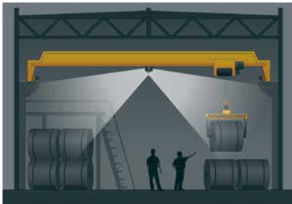
371LED/371LEDX is shipped from the factory with the standard reflector that creates a horizontal light beam that is 90 degrees from the vertical orientation resulting in a wide light output distribution.
