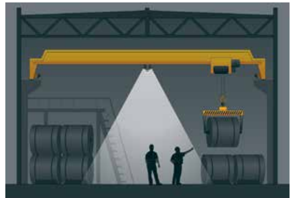
371LED with the 371LED-KIT-CR reflector installed reflects the light beam at 22.5 degrees from the vertical orientation resulting in a focused light output.
