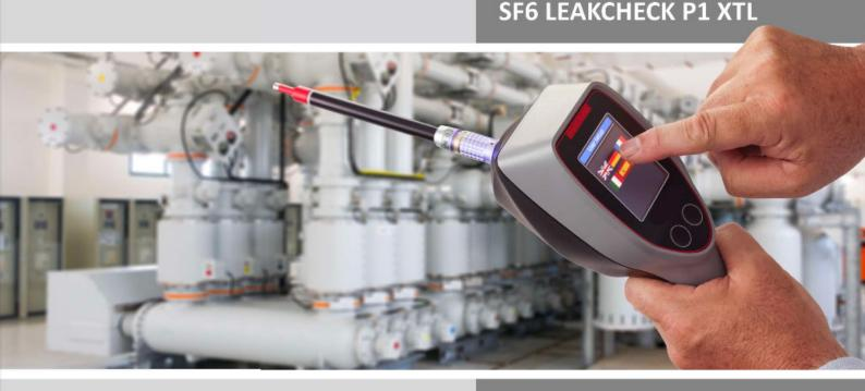
Once a leak has been localised, the push of a button puts the instrument into "Measuring Mode" if desired. In this mode the handgun display is switched to numerical reading. It is now possible to precisely measure the leak, with the leak rate displayed on the handgun screen.
