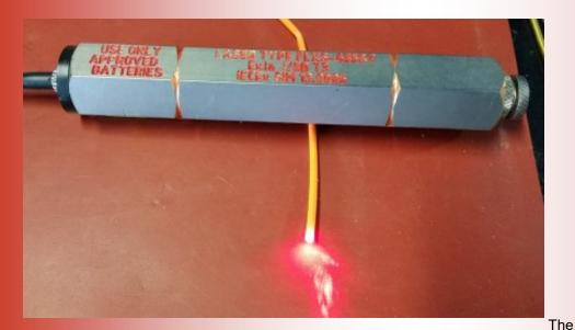
FLXS-635-ST is an Intrinsically Safe 5 milliWatt fibre coupled visible red laser for use with –ST type fibres. The product is also available with appropriate fibre couplings for use with –SC type fibres as the FLXS-635-SC
