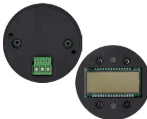
EA200-DisplayHousing Accommodates (1) Display PCB
