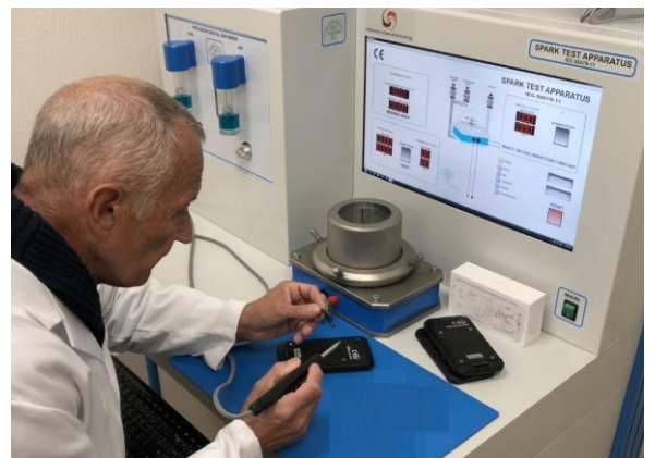
All devices are tested in the explosive atmosphere of the spark-test apparatus for intrinsically safe circuits
