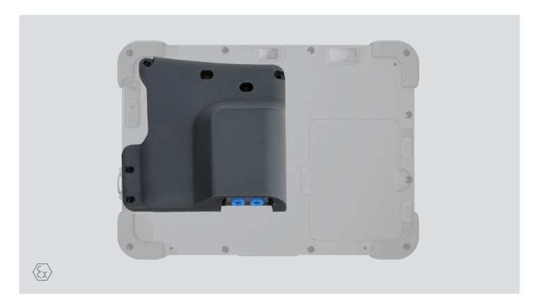
The HART Add-on Module is a new extension module for Agile X IS and offers a HART modem function. It may be connected to a HART loop as secondary master and facilitates applications such as configuring the HART devices.
