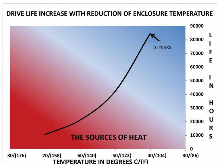
**Solar Load** When enclosures located outdoors are exposed to the sun, heat will be transferred to the inside of the enclosure. This is known as solar load or solar gain. (The effects of solar load can be significant; an automobile
