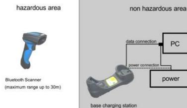
The Bluetooth handheld scanner can also be used separately in the hazardous area. The base or charging station is then operated in the non-hazardous area.
