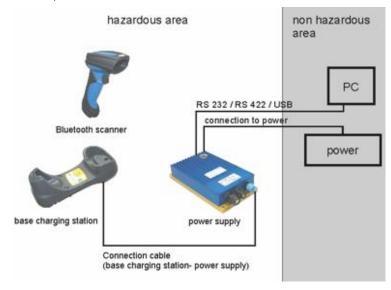
The Bluetooth handheld scanner was designed for use in hazardous areas. Normal operation requires a base station, a connection cable between base station and power supply, power supply, and connection cable(s) between power supply and a PC.
