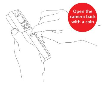
Install the batteries in the correct orientation (indicated on the enclosure) and close the lid again. PLEASE NOTE: Only those batteries listed in the Safety Instructions can be used.
