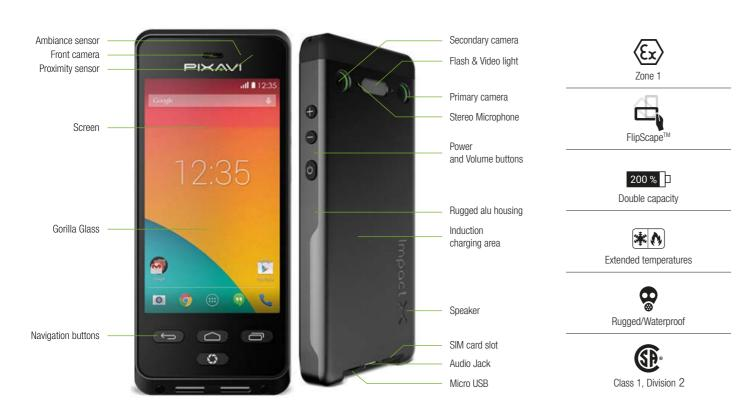
The BARTEC PIXAVI Impact X is the toughest smartphone you will ever meet. This intrinsically safe smartphone has all the functionality you will expect from a regular smartphone. The CSA, IECEx and ATEX certification has not compromised the quality and usability. The device is explosion proof and rated for use in hazardous areas. The Impact X is the next generation wireless video communication technology from BARTEC PIXAVI.
