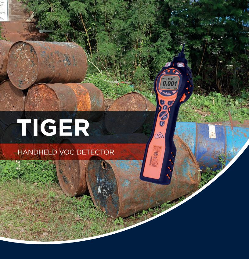
HUMIDITY RESISTANT PID TECHNOLOGY WITH ANTI-CONTAMINATION DESIGN
