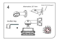
4. Tighten 6 x screws between arm and junction box, turn
