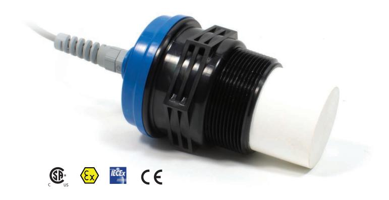
MNU IS ultrasonic sensors are rugged units, rated Intrinsically Safe for hazardous location installations. They feature APG's new QuickMode for power-saving, on-demand measurements, and optional GDT surge protection. All MNU IS sensors are fully programmable via RS-485 Modbus communications, and with APG Modbus software and an RS-485-to-USB converter.
