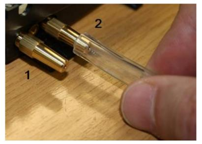
• The Zero and Span times are affected by the length of pipe between the gas source and the Calibration Dock. For best results, ION Science recommends that pipe lengths should be kept to a minimum; the shorter the length, the less gas is needed.
