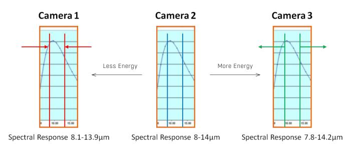
All three cameras "see" slightly different radiant energy levels for the same target temperature. The cameras all read the same as they are calibrated to "understand" that this specific level of intensity equates to a specific temperature, however this will cause an error when used with a spectrally transmitting IR Window.
