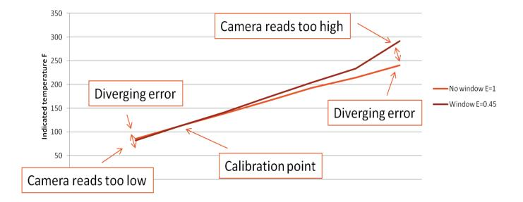
The graph above shows the effect of a single point calibration over a range. At the calibration point, the camera is accurate. However, as the same calibration factor is applied to increasing and decreasing target temperatures, significant errors occur.
