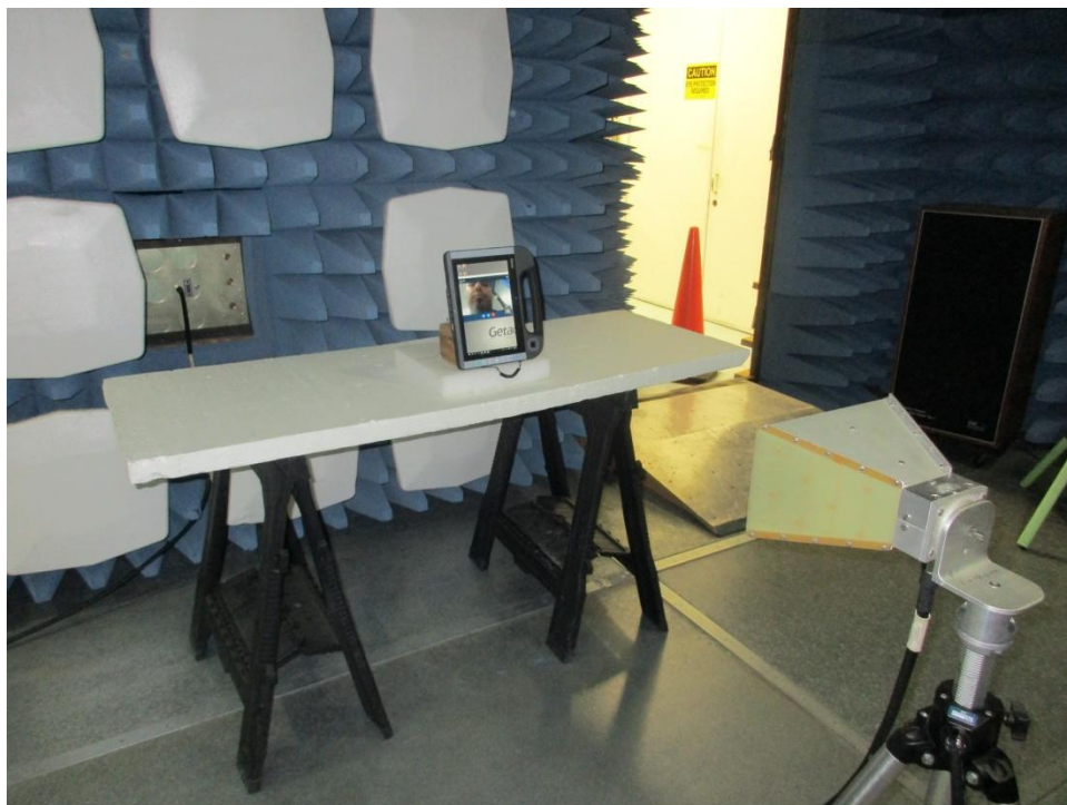
13 April 2016 -- HERO Wi-Fi Vertical-Face Edge 4 Down Getac Inc. Tablet, P/N RX10, S/N RG139R0076
