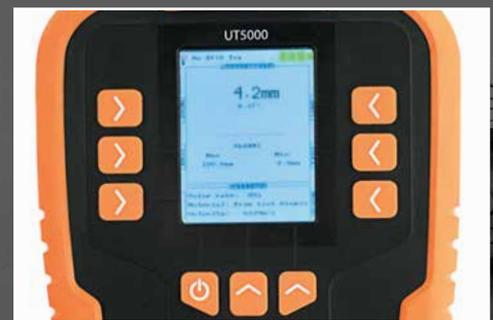
Menu "flip" function allows use by both left and right handed technicians.
