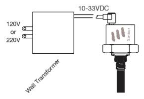
Operation with DC Power Supply Dew Point viewed on Instrument Display and available as 4-20mA output
