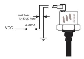
Operation with DC Power Supply Dew Point viewed on Instrument Display and available as Voltage output
