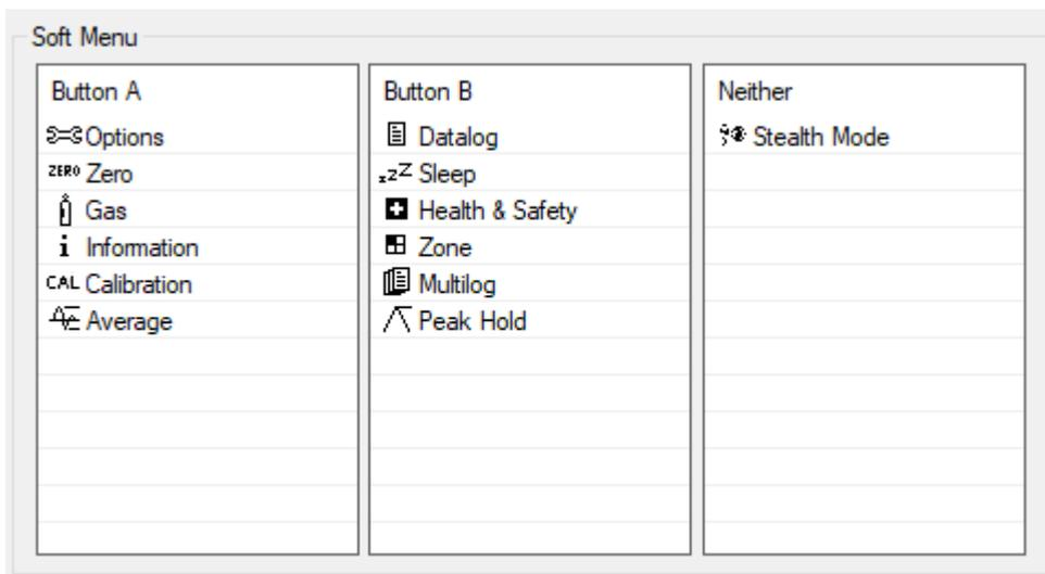
The various functions listed here may be allocated to the **A** and **B** keys (or neither) in any order by dragging and dropping them to the required positions in the lists. The order in which they are listed under a button controls the order in which they are listed in the soft-key menus.
