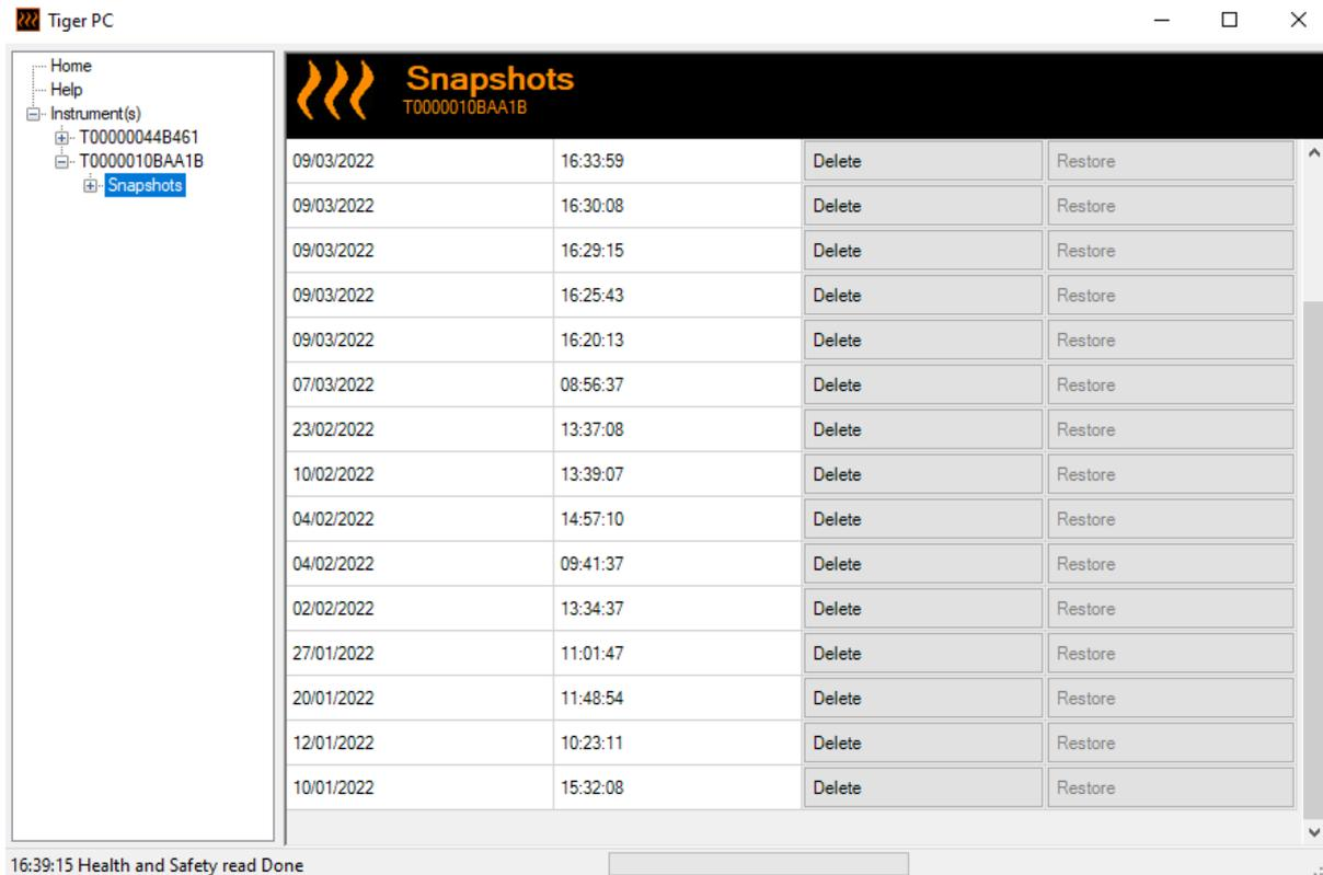
Details of a snapshot can be viewed by expanding the menu entry for that snapshot and accessing the Features, Summary, Configuration etc. screens for the snapshot:
