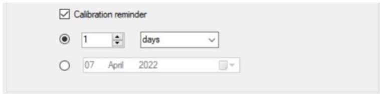
The calibration reminder allows you to set a reminder for when calibration is needed. To turn on the calibration reminder, ensure the box is ticked next to ‘calibration reminder’. You then have two options below that. You can either set how many days, weeks or months you want the reminder to appear after the day you are on, or you can set a more precise date by selecting the bottom option. The calibration reminder looks like the below.
