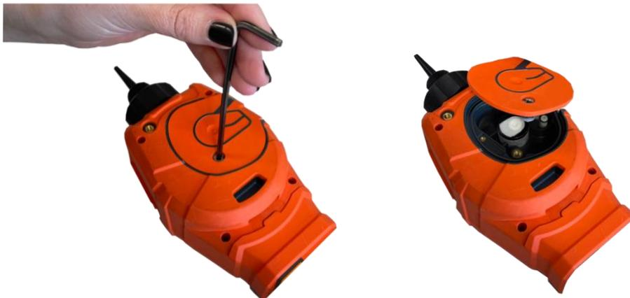
On the Sensor Cover loosen the bottom left screw using a suitable allen key.
