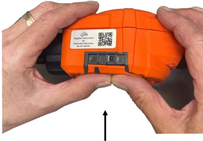
Once you hear it has engaged, push the rest of the sensor cover to the instrument body and screw the bottom left hand screw into place using the 3mm A/F allen key.
