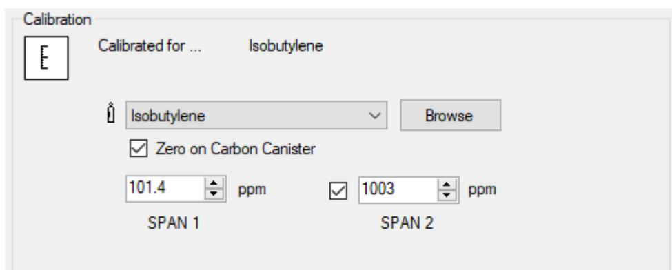
TIGER XT allows you to custom calibrate using any gas from the Gas Table at any concentration from 10 ppm. You will need a cylinder of the gas at the chosen concentrations.
