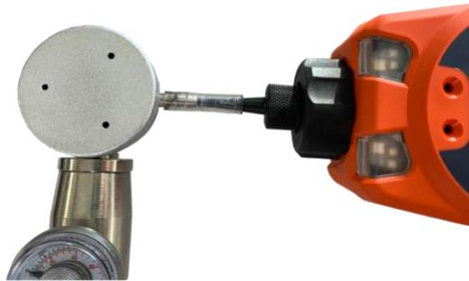
6. At the end of the countdown a tick '✓' will appear, indicating that the SPAN 1 has been accepted. Press **Enter**. For a two-point calibration, the calibration procedure is complete.
