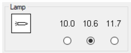
Enables the selection of different lamp types you may have purchased to use with your instrument. Ensure that the lamp selected is the same as that fitted in your TIGER XT. If not, select the correct lamp from the options provided.
