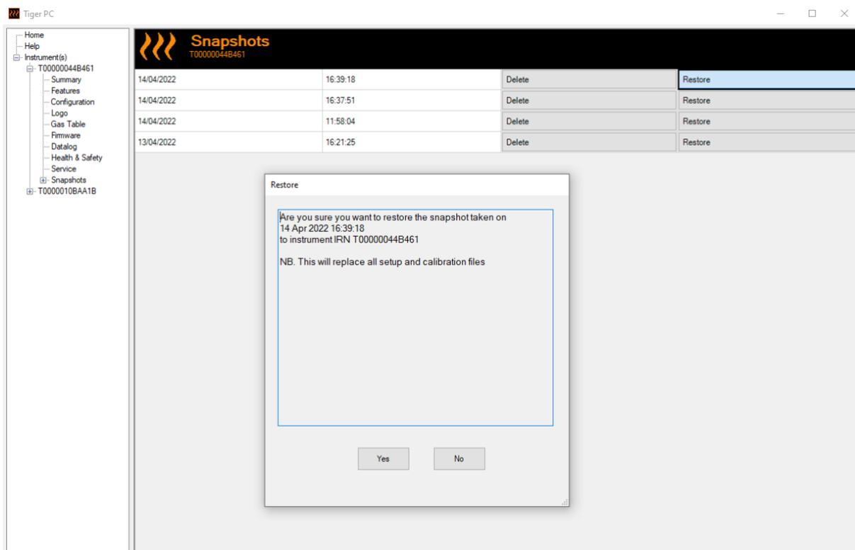
Click **Yes** to load the snapshot. When the loading is complete, click **Close** and restart your TIGER XT. Your TIGER XT will now be restored to the settings and calibration data stored at the time of that snapshot.
