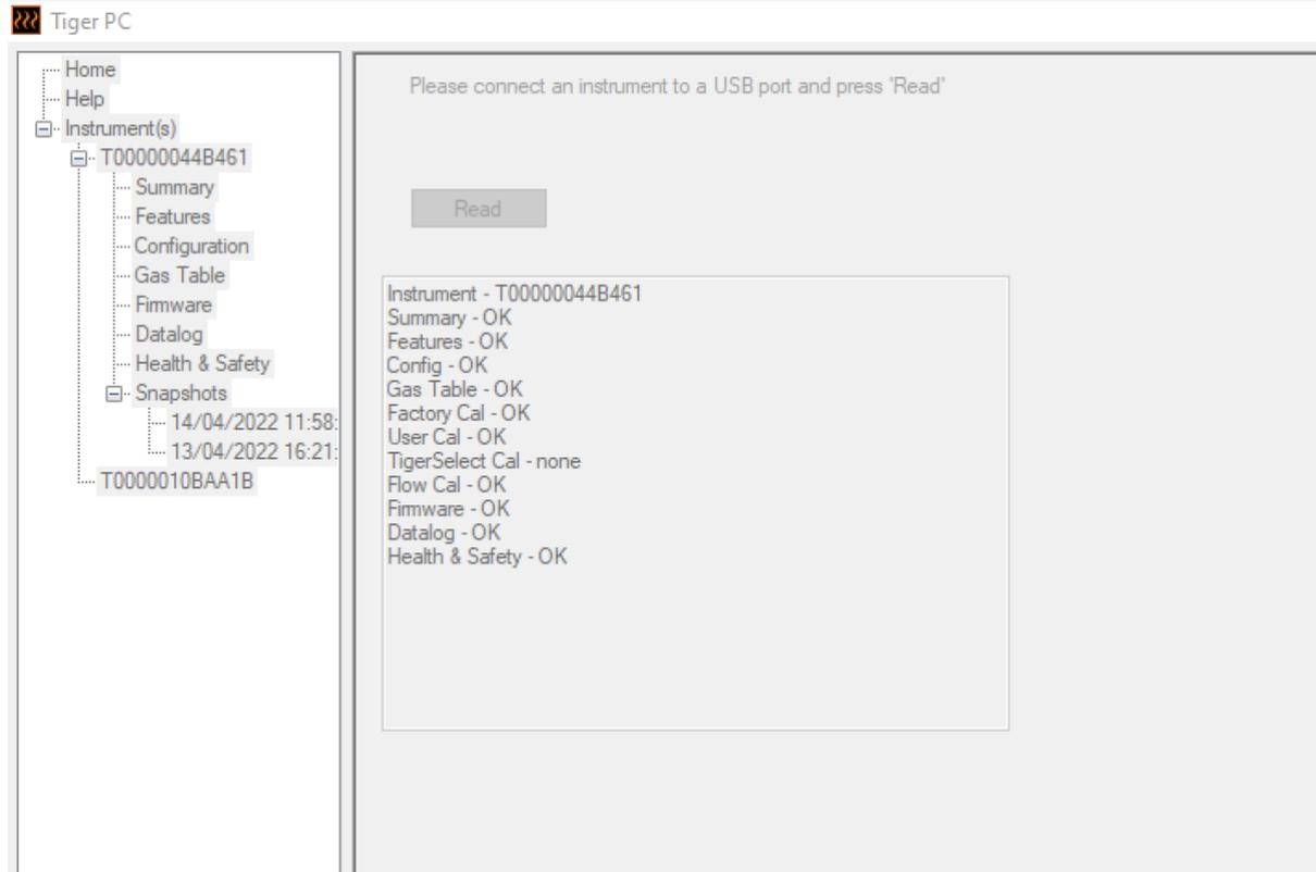
To remove an instrument from the list, click **Delete**. All details of the instrument are then removed from the software. If that instrument is connected again, it will be treated as a new (previously unlisted) instrument by TigerPC.
