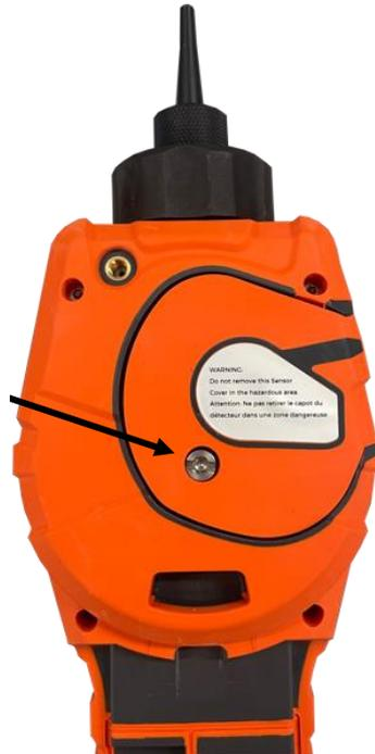
Once the screw is loose, gently pull the right side of the sensor cover from the instrument body until you feel that the sensor cover has unengaged from the inlet/outlet ports. Once it is unengaged, gently pull the entire sensor cover from the instrument body.
