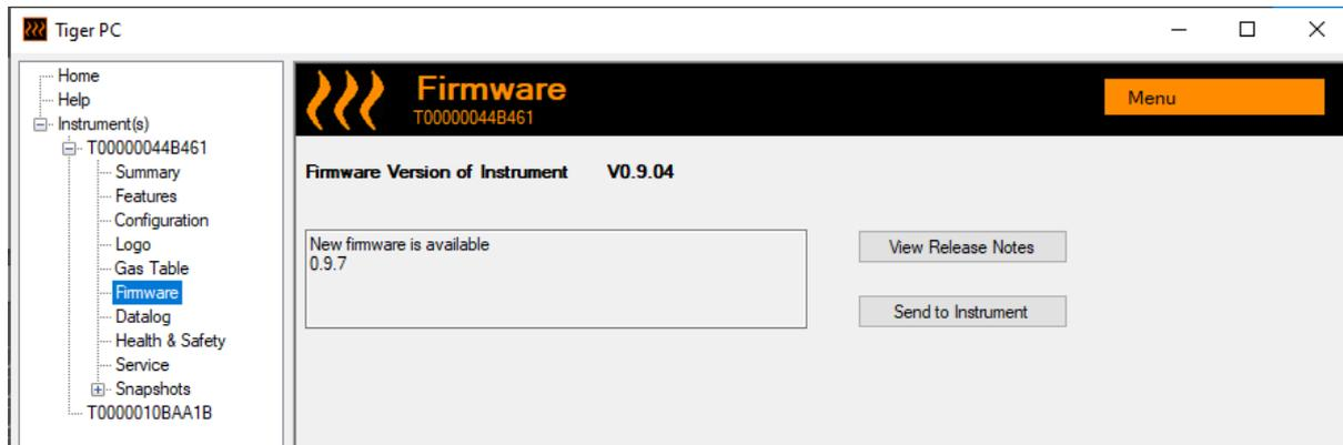
If new firmware is available, this will be noted on the screen in the box under the current firmware version: “New firmware is available”.
